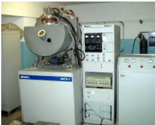
Fig. 1. View of vacuum-pumping assembly for ion plasma plating
